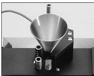
Macro bore funnel flow cell
